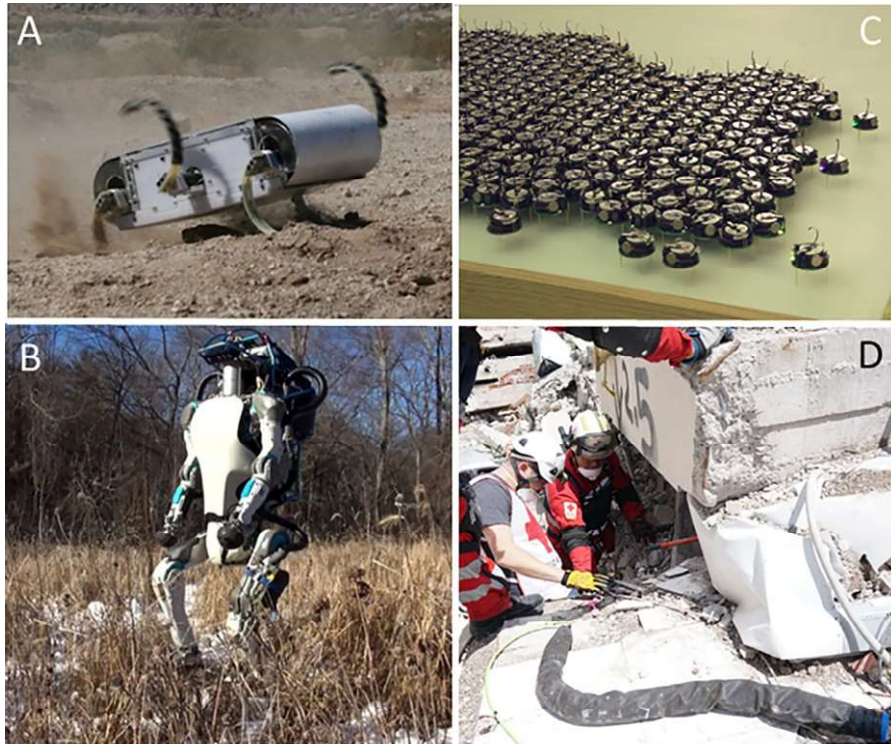
Fig. 6.1 Autonomous robots exhibit increased mobility on a variety of complex terrains. (A) Hexapod robot “RHex” moving over rough terrain; (B) Atlas, designed to operate outdoors and inside buildings; (C) “Kilobots” are programmed to exhibit complex swarming behaviors; (D) modular snake robot that was used in Mexico City earthquake to search for survivors. (A) credit: Kod*lab, University of Pennsylvania. (B) credit: Boston Dynamics. (C) credit: Self-Organizing Systems Research Group, Harvard University (D) credit: Biorobotics Laboratory, Carnegie Mellon University Robotics Institute.
